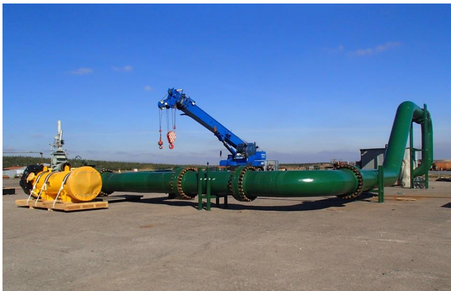
Figure 21: Offline Test Rig and Launch and Receive Vessel
